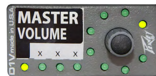
Figure 13: Use the Master Volume knob to control all audio outputs to the ePods. Note that this image depicts maximum volume.
