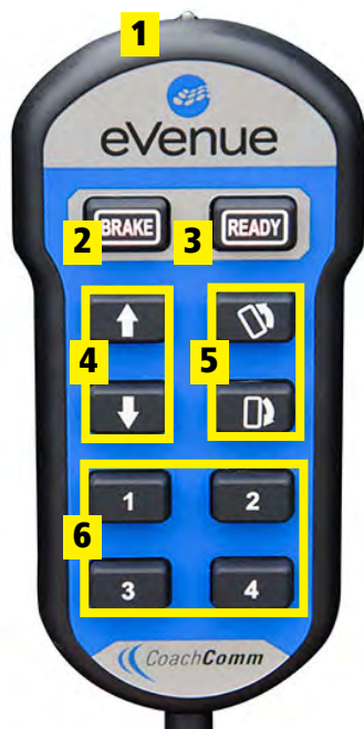
Figure 22: Use the Commando-e Remote to control the ePod's Motion Control System.
