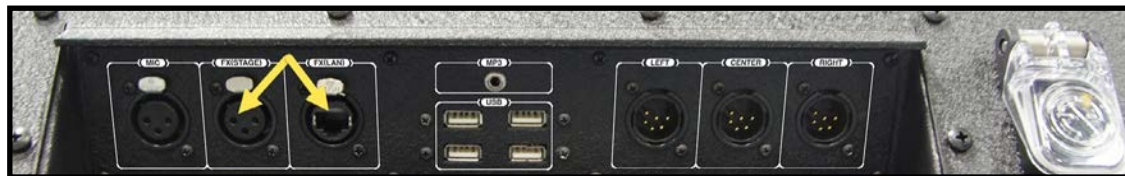
Figure 17: Tempo Go's Control Unit connections for a Tempest FX BaseStation
