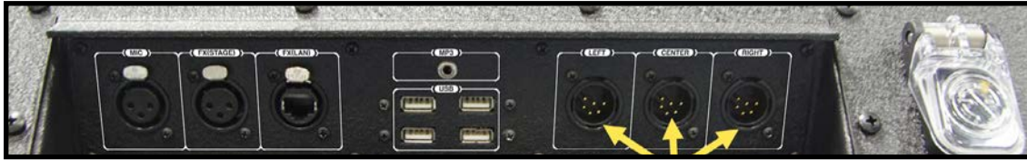
Figure 22: I/O Connection Panel Output to Speaker Connection
