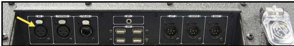
Figure 16: Tempo Go's Control Unit connections for a microphone
