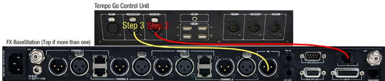
Figure 15: Tempest FX BaseStation Cables to Tempo Go Control Unit
