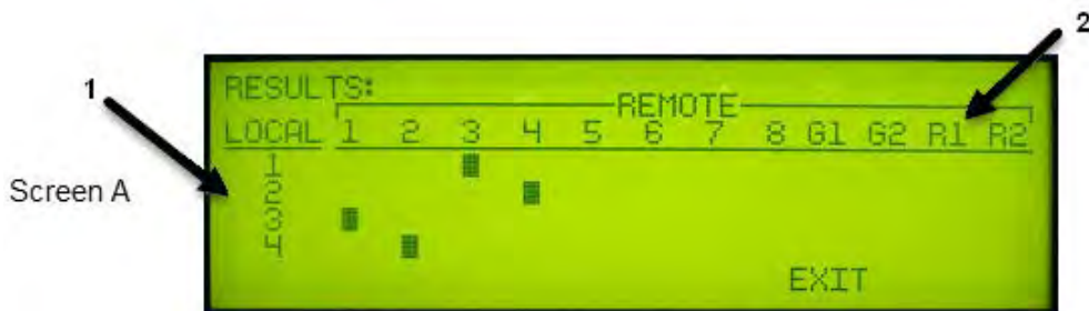
Figure 33: WIM 8 Dry Pair Testing Fault Screen
