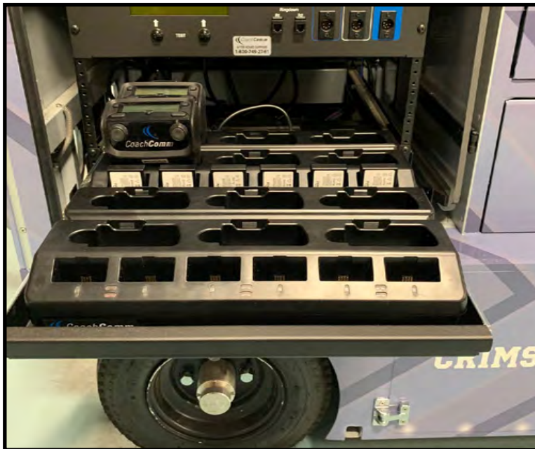
Figure 54: 6+6 Drop-In RP and Battery Chargers
