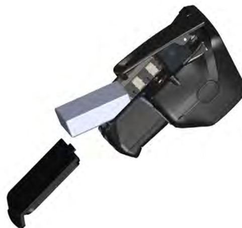
Figure 56: Radio Pack Battery Installation
