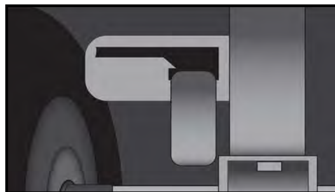
Figure 25: Second-Generation Cart Brake Lever Position for Manual Towing
