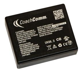
The rate of degradation of Lithium-Polymer batteries is strongly temperature-dependent; they degrade much faster if stored or used at higher temperatures. Elevated temperatures (whether from charging or ambient air) hasten capacity loss. Poor ventilation may increase temperatures, further shortening battery life.
